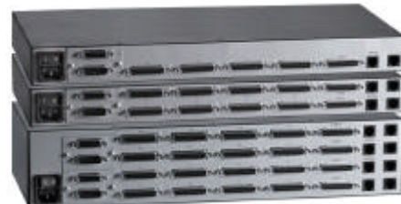
UltraMatrix Remote rear panel 1x4, 2x8 and 4x16 (Shown with optional expansion cards installed)
